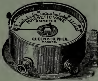
"Magnetic Vane" Ammeter.
