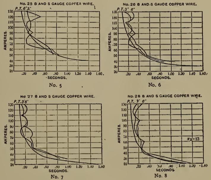
range, but in the larger size wires, a greater current was required to fuse the wires in the 1.5 second limitation, consequently the curves given for the larger fuse wires show less and less range as the fuse wires increase in size.
