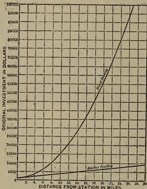
DIAGRAM 1.—INITIAL COST OF STEAM AND GENERATING PLANT, COPPER AND SPECIAL APPARATUS FOR DELIVERING 200 AMPERES AT 500 VOLTS.
