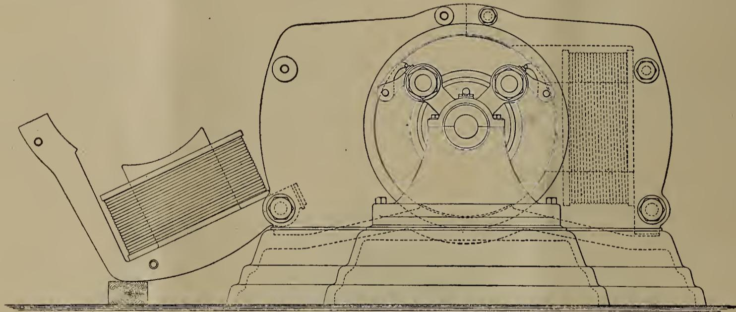
FREEMAN DIRECT CURRENT DYNAMO—REMOVED FIELD COIL.
