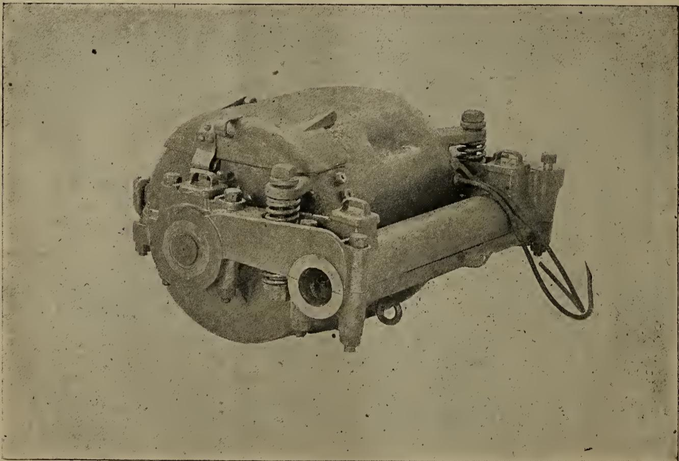
FIG. 1.—WALKER MFG. CO'S FOUR-POLE SINGLE REDUCTION STREET MOTOR.
