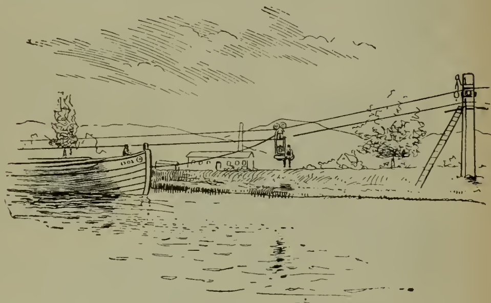
ELECTRIC POWER HAULAGE FOR CANAL BOATS.
