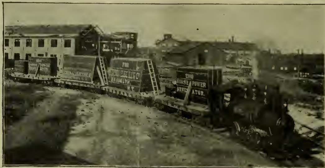
Fig. 3. Four of Five Cars, Loaded with Brooklyn Generator Only.
