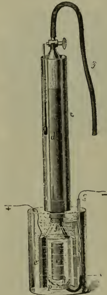
Volume Voltmeter, for Measuring Current.
