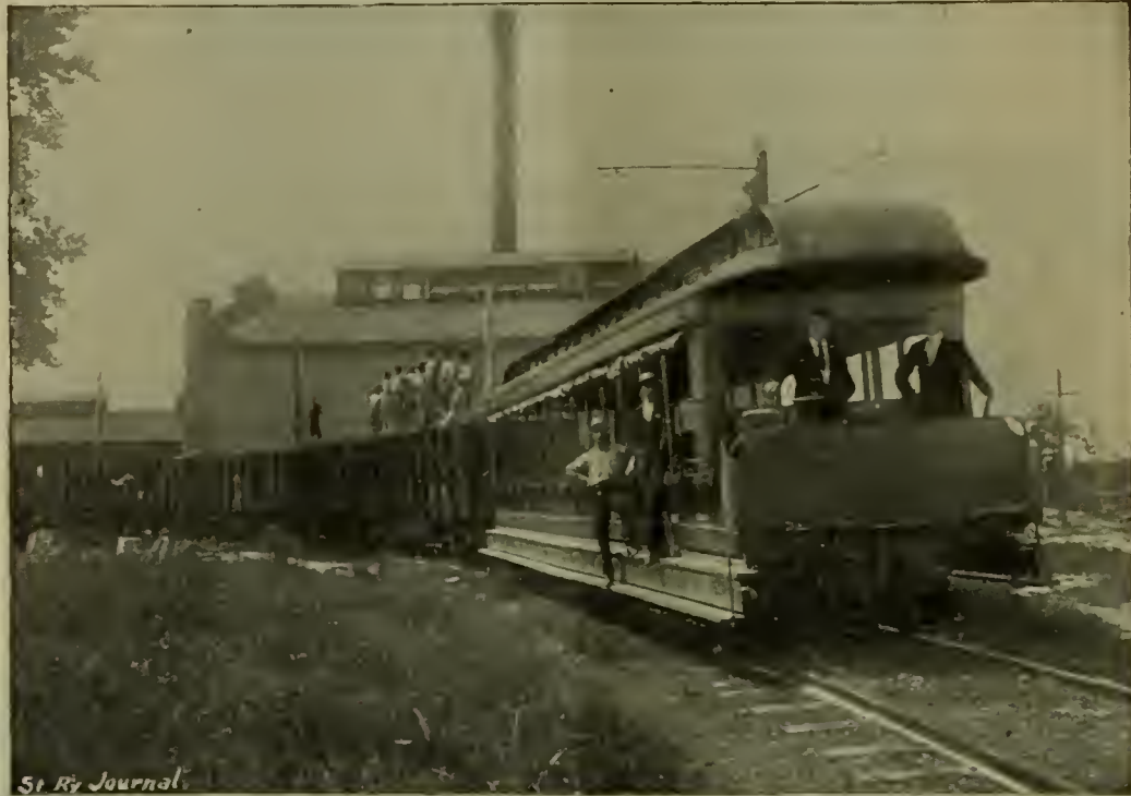
Fig. 8. Motor Car, Equipped with Walker Co. Motors, Drawing Loaded Freight Train.
