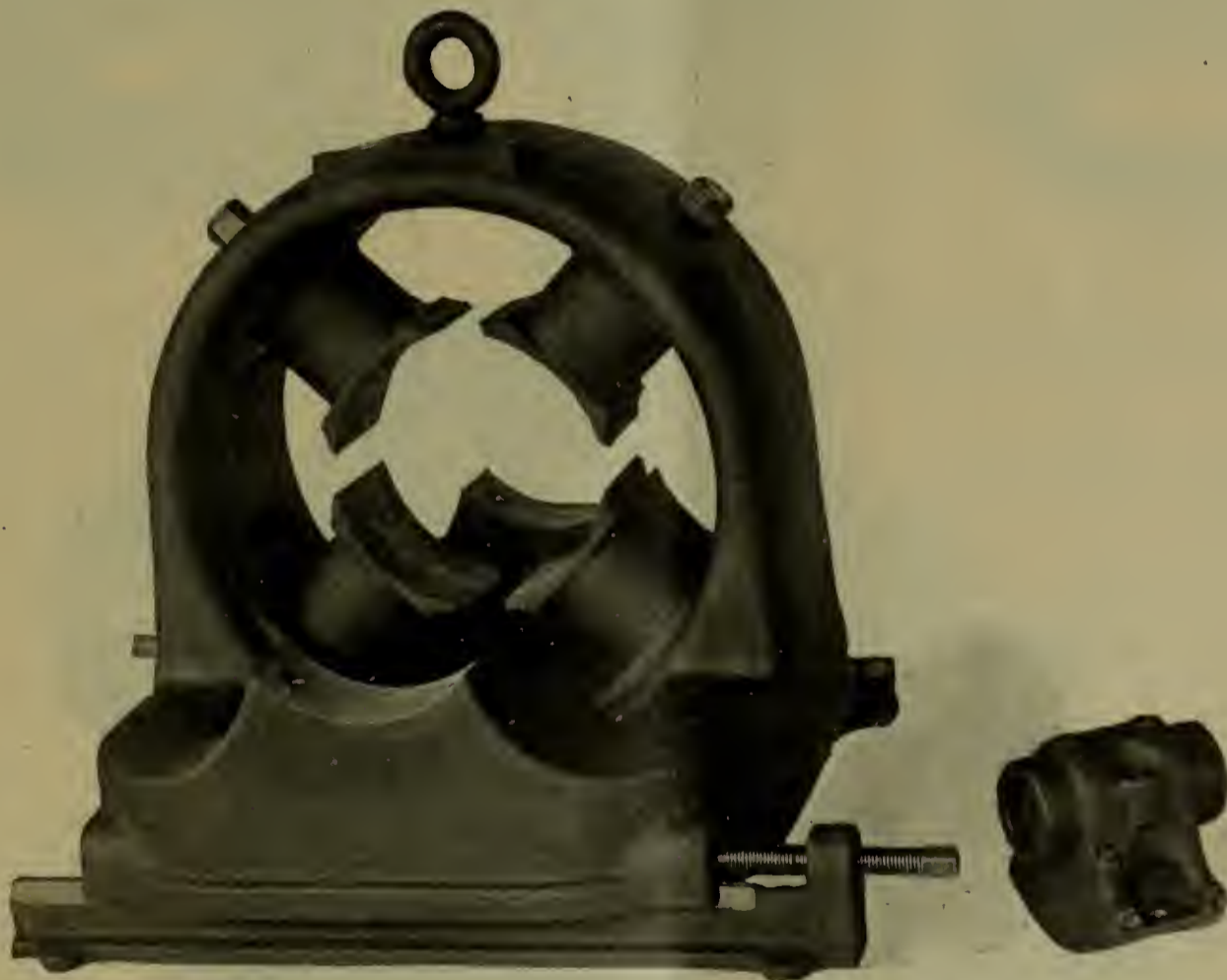
View Showing Frame Construction. (Walker Elec. Mfg. Co.)
