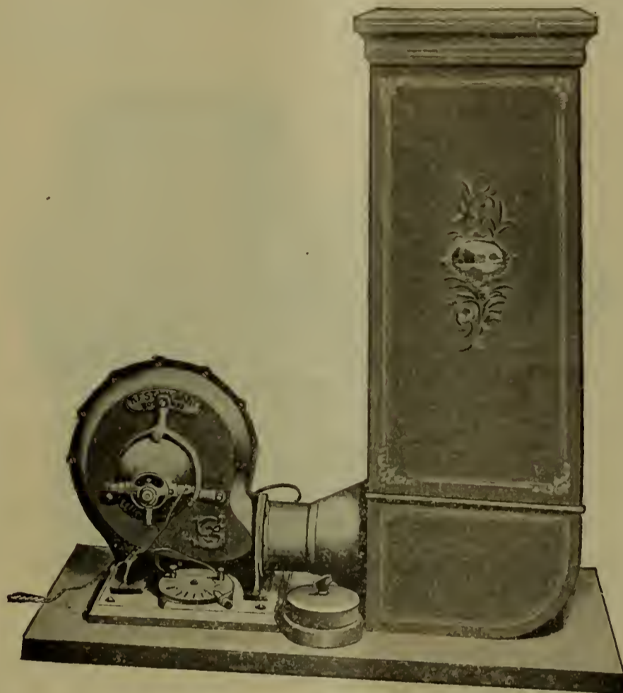
Lundell Motor, Sturtevant Blower and Gold Heater Combination.—Hot Blast System of Electric Heating.
