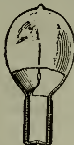
LAMP WITH ONE FILAMENT, ONE INSIDE AND ONE OUTSIDE CONDENSER COATING, AND AUXILIARY COATING.
