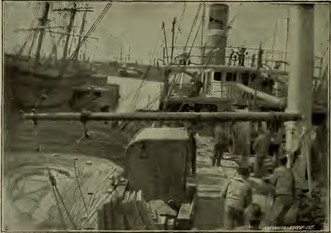
UNITED STATES CABLE SHIP "HOOKER."—VIEW LOOKING AFT FROM FORECASTLE, SHOWING "SAFETY" CABLE BEING RECEIVED ABOARD FROM SCOW AND COILED IN TANKS—THE MEN IN THE FOREGROUND ARE SPLICING TOGETHER TWO LENGTHS OF "SAFETY" CABLE.
