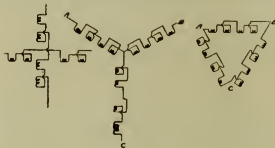
FIG. 1.—TWO-PHASE; THREE-PHASE STAR, OR Y; THREE-PHASE DELTA CONNECTION.
