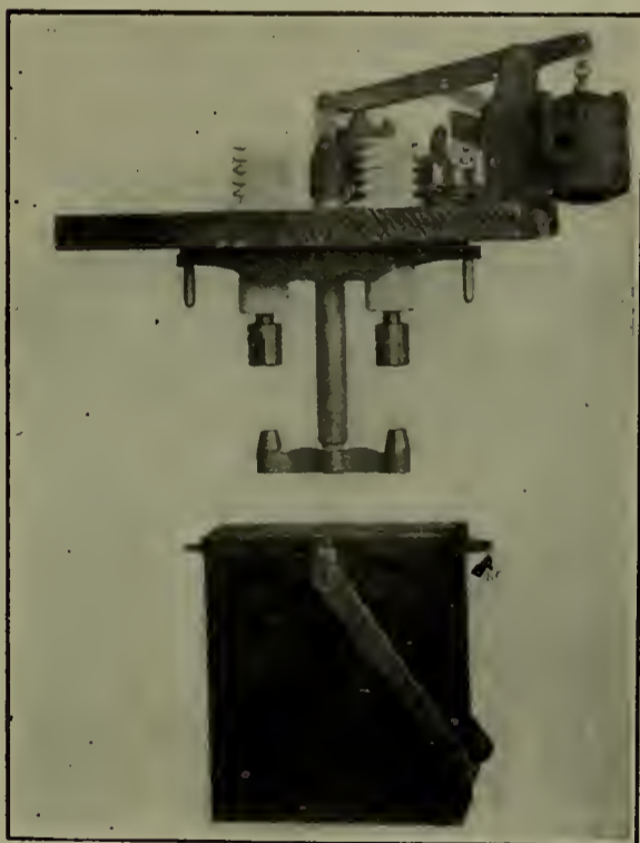
FIG. 13.—SMALL SOLENOID-OPERATED OIL CIRCUIT-BREAKER.
