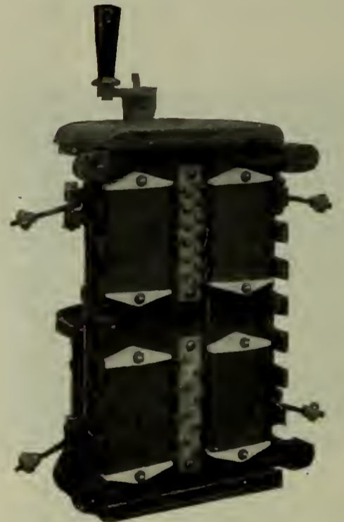
Fig. 2. REAR VIEW (BACK PLATE REMOVED) SHOWING SHUNT FIELD RESISTANCE UNITS MOUNTED ON BACK OF CONTROLLER.
