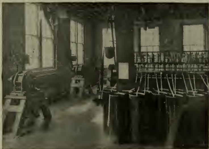
FIG. 2.—TWO 10 H.P. 220 VOLT KG SINGLE-PHASE MOTORS DRIVING A SEPARATE LINE SHAFTING, FROM WHICH ARE DRIVEN CARDING MACHINES, DRAWING FRAMES, ROVING MACHINES AND FLY FRAMES.
