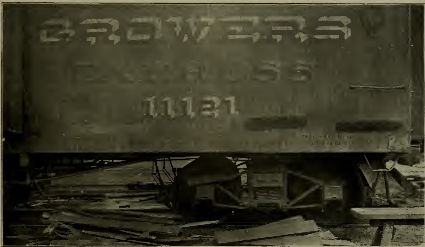
IMPROPER METHOD OF STENCILLING THE CAPACITY AND LIGHT WEIGHT UPON CARS.
