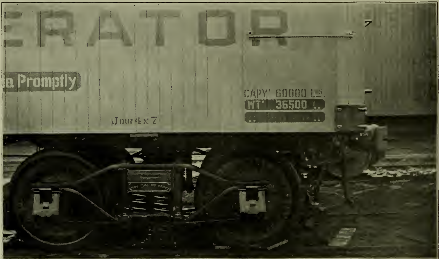
PROPER METHOD OF STENCILLING THE CAPACITY AND LIGHT WEIGHT UPON CARS.
