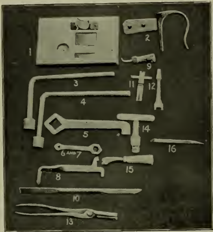
MR. HARVEY'S AIR BRAKE TOOLS.—DETAIL DRAWINGS OF THESE WERE GIVEN IN OUR LAST ISSUE.
