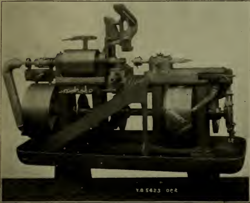
PRATT & WHITNEY CO. EXHIBIT—No. 14. AUTOMATIC SCREW MACHINE.
