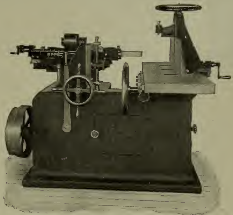
S. A. WOODS MACHINE CO.'S NO. 6 HORIZONTAL HOLLOW CHISEL MORTISER.
