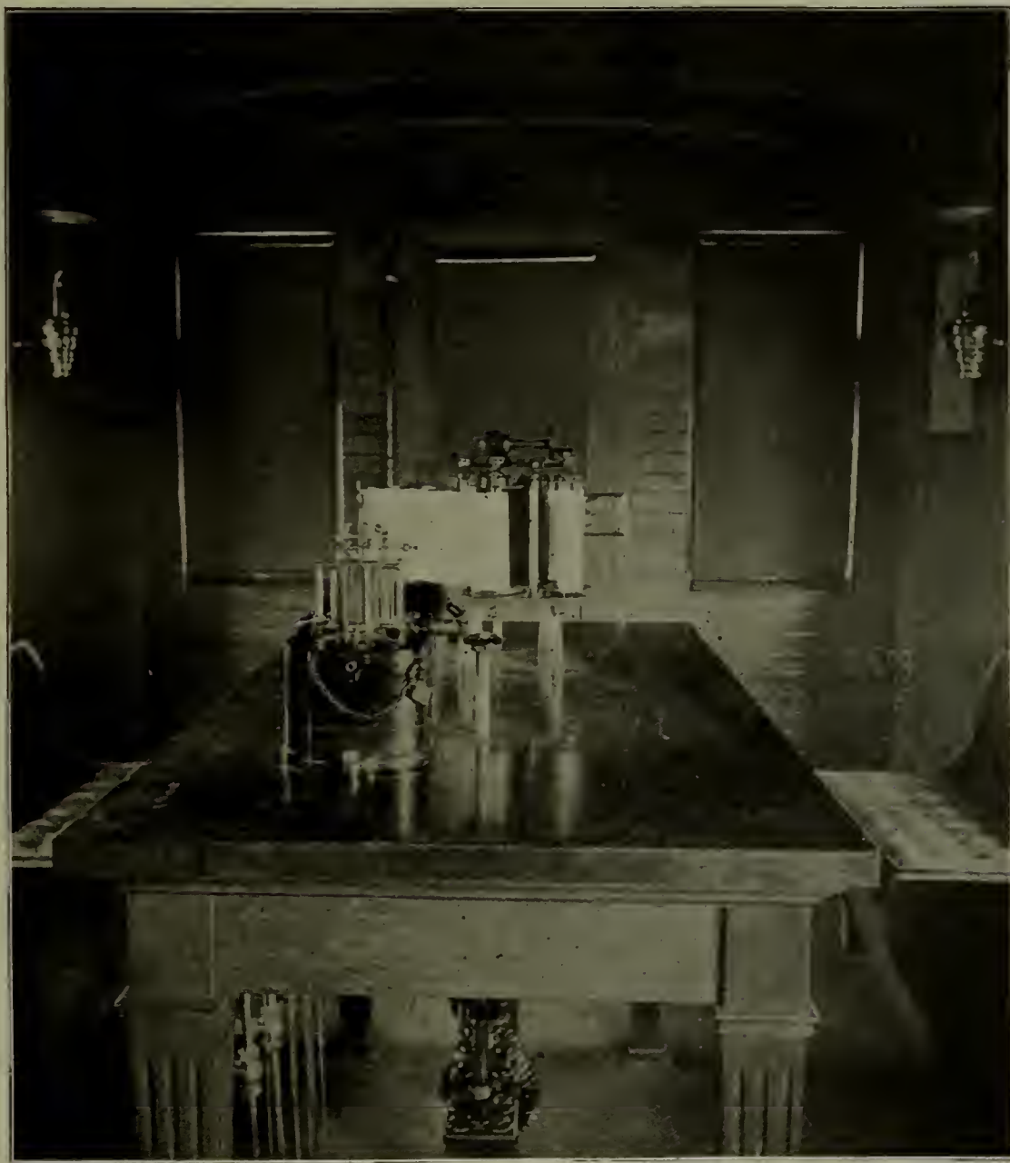
TEST CAR NO. 17, FIG. 5.—APPARATUS FOR MEASURING TRAIN RESISTANCE.
