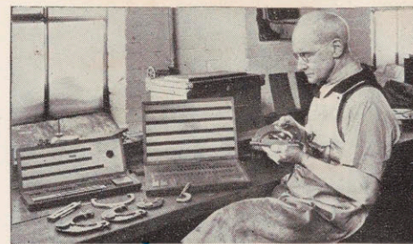
Coppus inspector checking master gauge with Johansson size blocks. All important dimensions are machined accurately to one-quarter of one-thousandth of an inch (.00025). Even dimensions such as center height (center line of shaft to bottom of turbine feet) are accurate to .002". All holes are drilled to jigs for interchangeability of parts.
