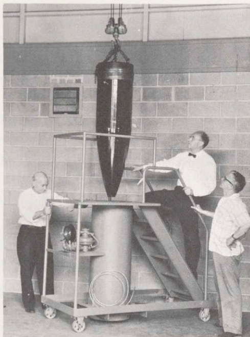
Fig. IX-2. Mobile mount for pressure-testing facility; pressure cylinder is shown suspended from crane.
