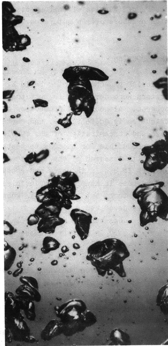
Figure 1b The air flow is 0.05 cubic feet per minute per orifice and the water flow is zero.
