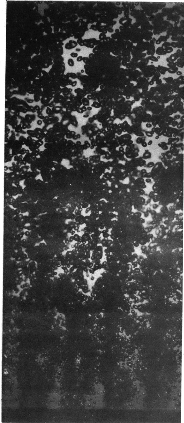
Figure 4b The air flow is 0.083 cubic feet per minute per orifice and the water flow is 0.1 gallon per minute per orifice.
