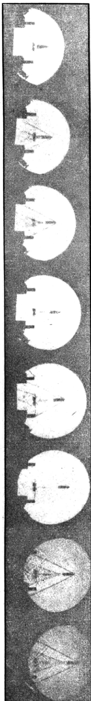
Figure 54 - Strip of Film Showing a Projectile Fired through a Strip of Copper; Image Frequency 100,000 per Second
