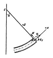
On a meridional section through P there act analogous stresses of resultant  ${\bf T}_2$  and the moment  ${\bf G}_2$  per unit length. Here the symmetry is lacking because of the shear.
