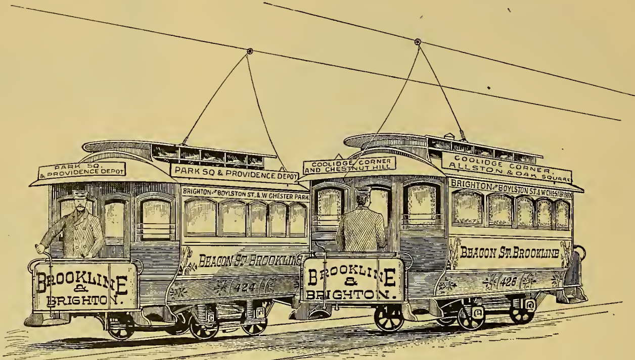
THE SPRAGUE ELECTRIC CARS ON THE BEACON STREET DIVISION OF THE WEST END ROAD. (By courtesy of The Beacon , Boston, Mass. From an illustrated article published by them Nov. 24th.)
