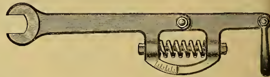
WRENCH FOR PRODUCING AND MEASURING FRICTIONAL ADJUSTMENT OF RINGS.
